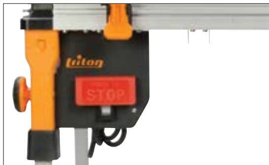
Mains isolator switch fitted for use with power tools
